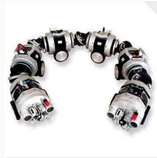
Inline inspection systems to get extensive information and data on distribution lines
